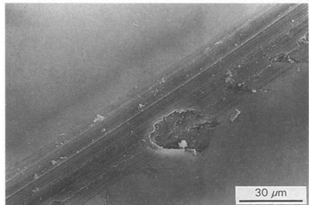
Figure 15 Secondary scanning electron micrograph (30 kV) of a 500 g scratch in 1 \times 10^{16} Y ions \text{cm}^{-2} implanted ( 10\bar{1}2 ) sapphire. A region of surface has adhered to the scratch diamond and has been pulled out of the specimen surface as the diamond passes, because the interfacial shear strength is larger than the shear strength of sapphire.
